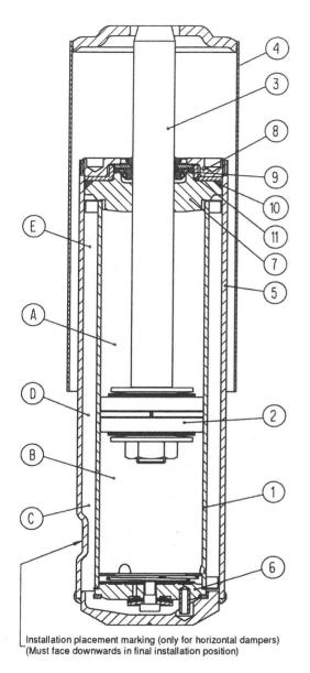
The piston (2) divides the pressure cylinder (1) into an upper and lower working chamber (A) and (B). In rebound, i.e. when the piston rod (3) extends, as well as in compression, damping forces are generated by the pressure differential between working chambers (A) and (B) above and below the piston. Pressure levels in the working chambers adjust automatically depending on piston velocity, and resistance to flow is controlled by the valves on the piston (2) and the base valve assembly (6).
