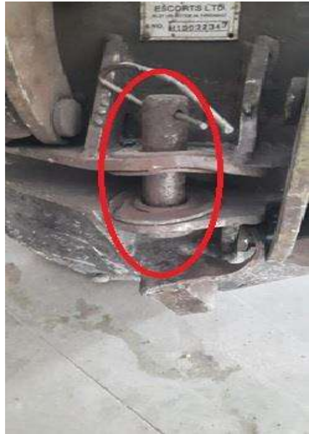
Fig (iv) - Use of non-standard bell crank lever pins
