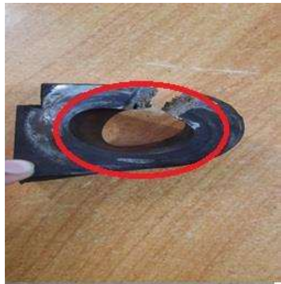
Fig (ii) - Bell crank lever with oblong hole
