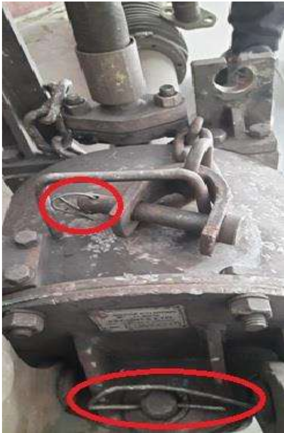
Fig (iii) - Improper locking of bell crank lever pin instead with standard spring dowel sleeve with bush arrangement
