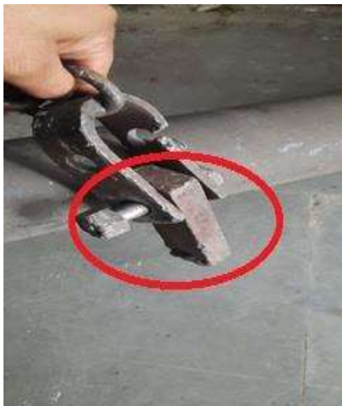
Fig (i)- Improper welding of U- clamp safety bracket for brake cylinder hanging
