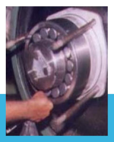
**AXLE BOX BEARING USED IN ICF BOGIE** Steps of Attention in POH (Contd...) Mounting Labyrinth Ring Heating upto 100°C Place on Shoulder Seat of Axle Pushing by Pusher Jig Light Tapping to ensure proper seating **Coating of Grease Rear Cover** Renewal of Felt Seal **Renewal of O-Ring** Ring
