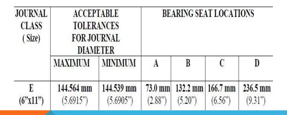
**AXLE BOX BEARING USED - CASNUB** Steps of Attention in POH (Contd...) Mounting Pressing of CTRB **Application of Rust Preventive Coating** On exposed surface of Axle **Between Hub and Bearing** Application of Thin Coat of Anti Slip Oil (SAE 40 or 50)
