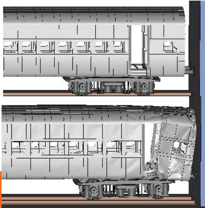
Baseline GS coach crush behavior with side buffers.
