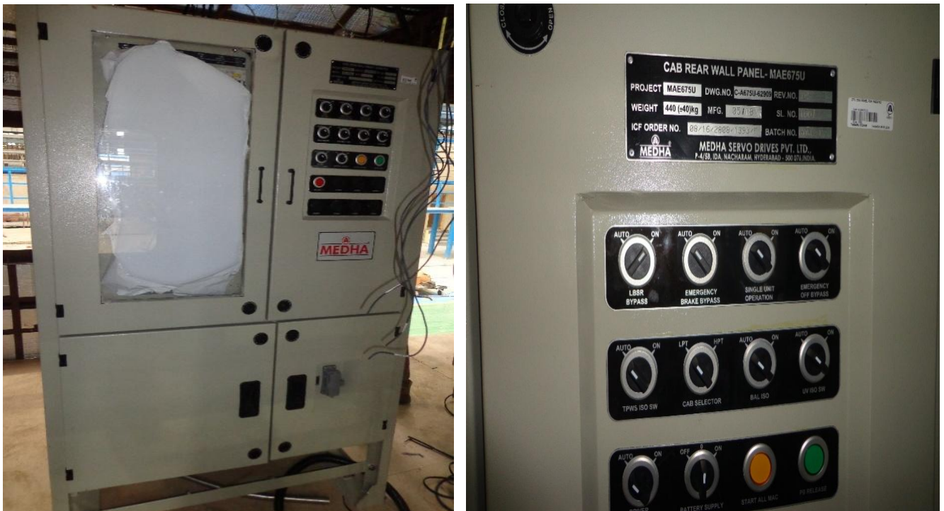
Fig8.0a: Cab Rear Wall (CRW) Panel
