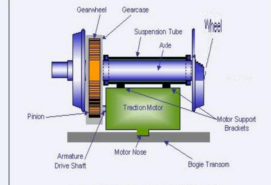
Diagram of DC Nose Suspended Traction Motor
