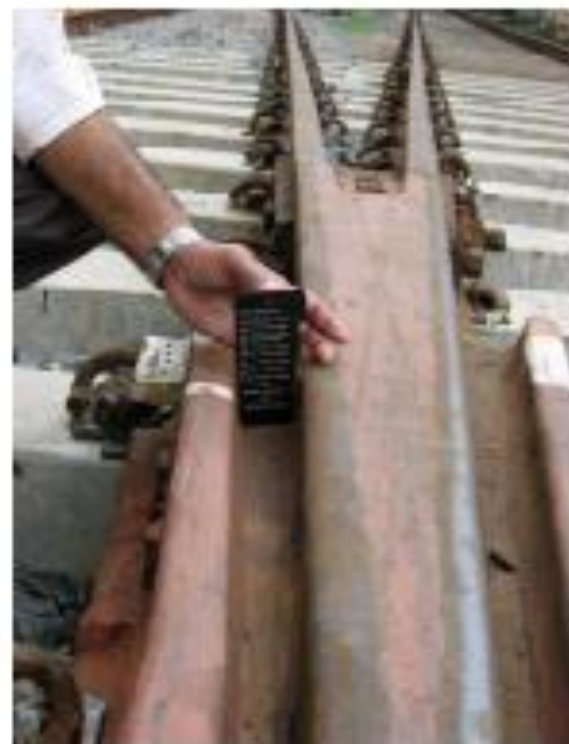
'Go-No go' gauge for measuring wing rail, check-rail clearance
