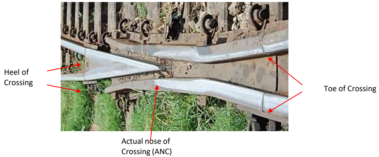
Cast manganese Steel (CMS) Crossings
