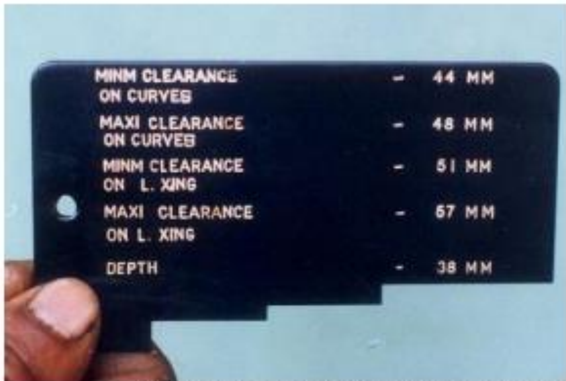
'Go-No go' gauge for measuring wing rail, check-rail clearance
