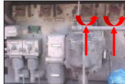
BC Isolating Cock (FTIL) (To move anti-clockwise by 90°)
