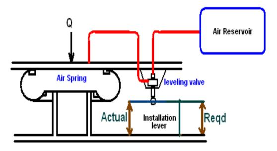
It connects the main reservoir with Air spring and admits more air, whenever the bolster comes down due to abnormal increase in the Pay load (Super Dense Crush load).
