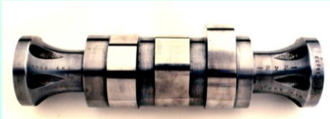
OLD FLANGE DESIGN WITH 6 HOLE DESIGN OF CAM SEGMENT
