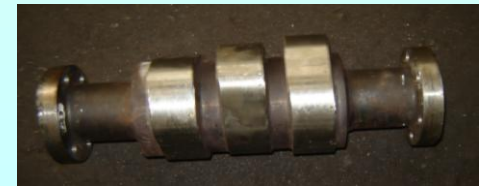
REVISED FLANGE DESIGN WITH 8 HOLE DESIGN OF CAM SEGMENT
