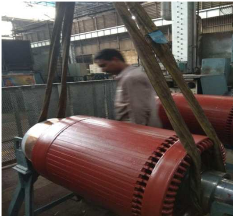
Lifting rope touching with Armature coil Evolutes
