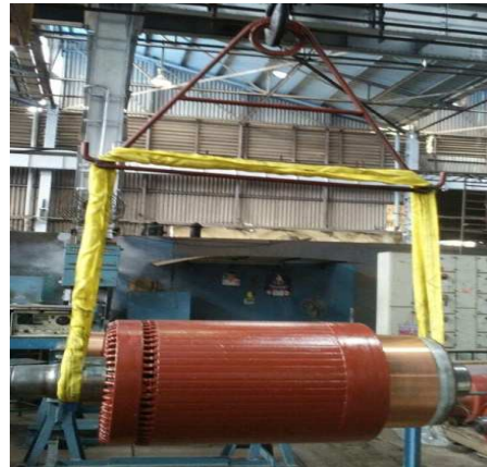
Gap is ensured between lifting rope and Armature coil Evolutes
