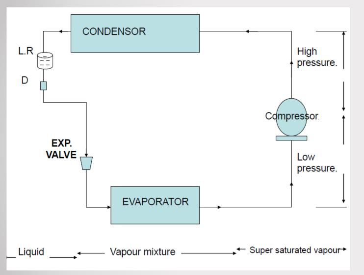
• The super saturated vapour refrigerant is cooled down to liquid state in the condenser by loosing heat to the atmosphere, thus completing the cycle.
