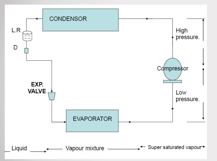
The vapour mixture (liquid + vapour) passes through the evaporator, where it absorbs heat from the control volume and gets converted to saturated vapour.
