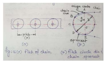
Pitch circle diameter: It is the diameter of a circle on which the hinge centers of the chain lie, when the chain is wrapped around a sprocket as shown in fig. 16(b)
