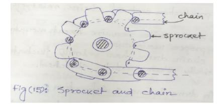
The toothed wheels are known as sprocket wheels or simply sprocket. The chain are mostly used to transmit motion and power from one shaft to another, when the distance between the centers of the shafts is short such as bicycles, motor cycle etc.
