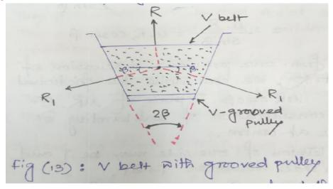
As per the fig, we can understand the construction of V-belt with grooved pulley.
