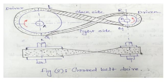
The belt RQ  $\rightarrow$  tight side & LM  $\rightarrow$  Slack side. To avoid the rubbing at the crossing point, the shafts should be placed at a distance of (20 X b), where b = width of belt and speed of belt should be less than 15m/s.
