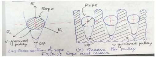
The fiber ropes are usually circular is cross section as shown in fig. The sheave for fiber ropes shown in fig. 14(b). the groove angle of the pulley for rope drives is usually 45°. The groves in the pulleys are made narrow at the bottom and the rope is pinched between the edges of the V-groove on the pulley.
