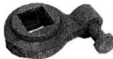
BROKEN ADJUSTABLE BUSHING
