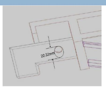
Remove Brake Head and inspect Brake Head pin hole in Beam. If hole exceeds 20.32 mm in length, replace Beam. If not, replace brake head and recheck tip as described earlier. Tip should not exceed 31.75 mm (from FIRST check above). If tip does exceed 31.75 mm, replace Beam and Brake Head.
