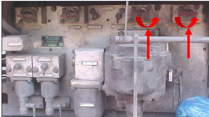
BC Isolating Cock (FTIL) (To move anti-clockwise by 90°)
