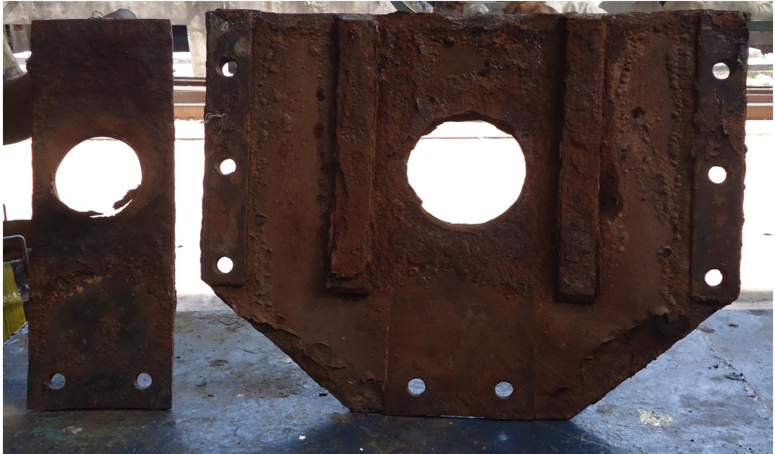
Central pin base plate and axial stiffener plate shown separately. The punctured hole on axial stiffener plate matching with existing hole on base plate allowing central pin to drop down wards causing coupler body to come out and parting.
