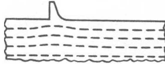
Force flow around a narrow projection: Low stress concentration.
