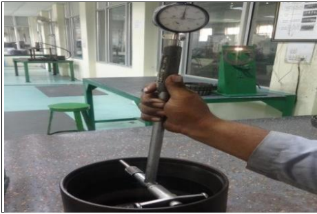
Fig.: Checking seal fit counter bore with dial bore gauge (recommended method)
