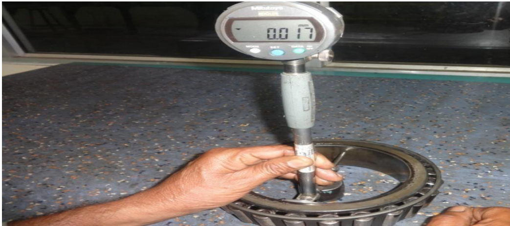
Checking inner ring bore with dial bore gauge (Recommended method)
