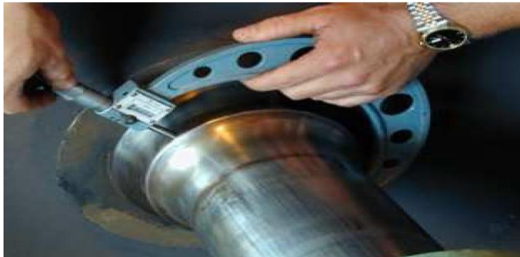
Fig. 45: Checking backing Ring Seat on Axle
