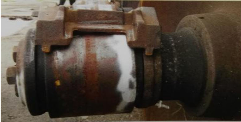
Fig.14: Damaged Backing Ring
