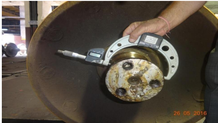
Fig. 49: Measuring journal diameter by snap gauge
