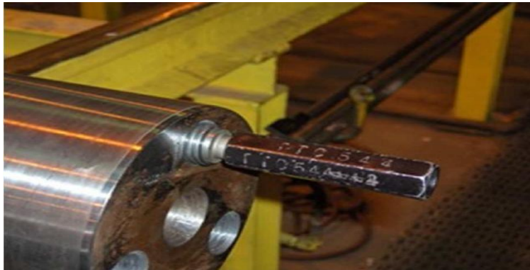
Fig. 46: Axle end thread checking Gauge
