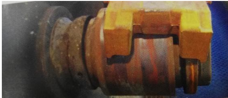
Fig.11: Damaged End Cap
