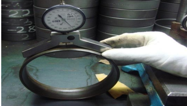
Fig: Checking Seal wear ring groove depth
