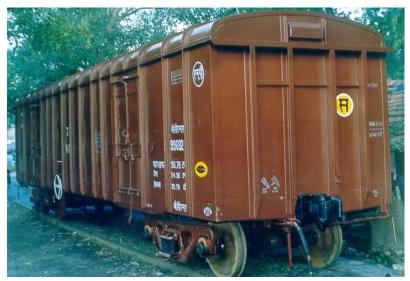
BCN- Bogie Covered Wagon (Riveted construction) fitted with Air Brake and CBC .
