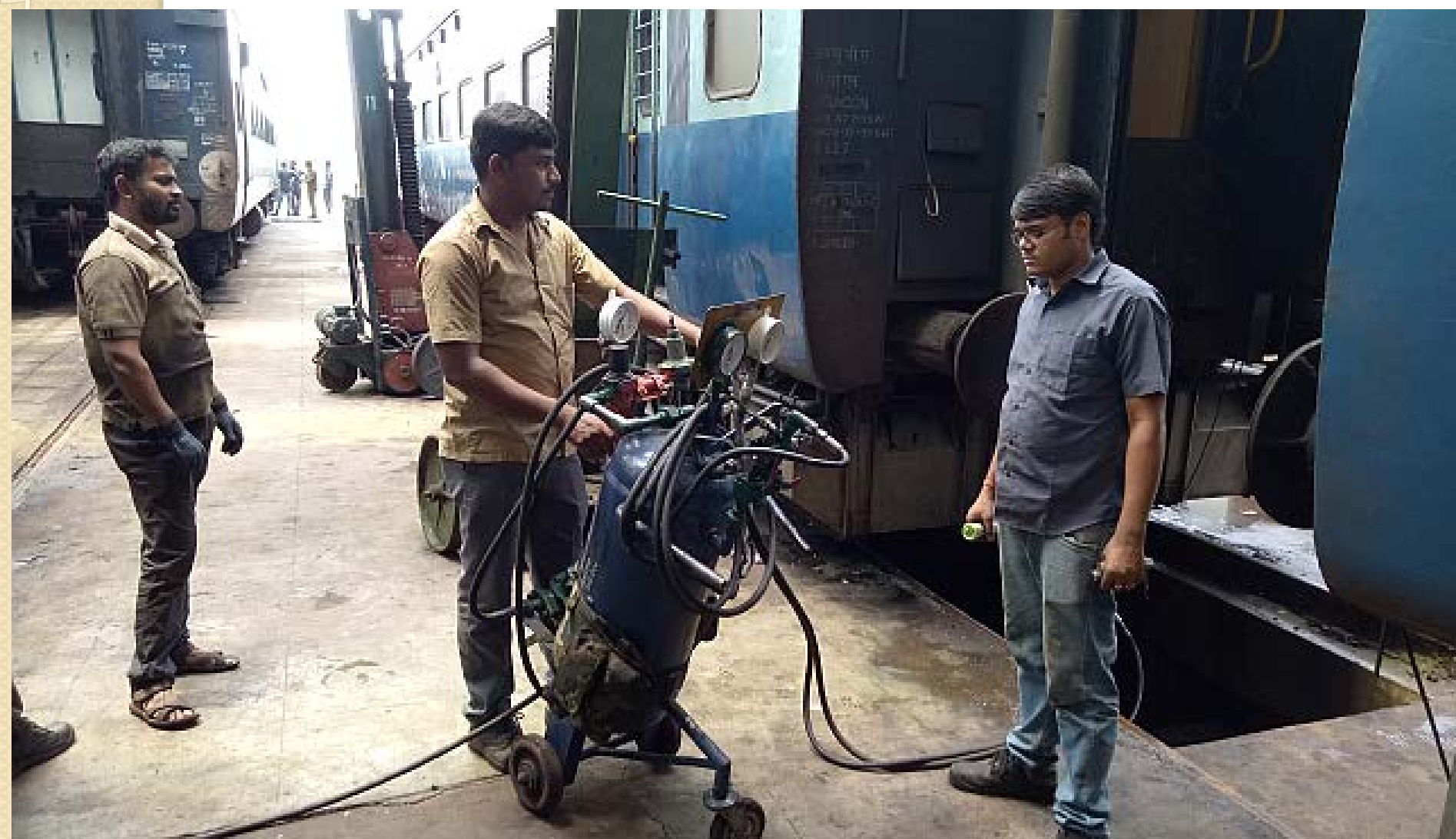
Testing of ready coach with single car test rig
