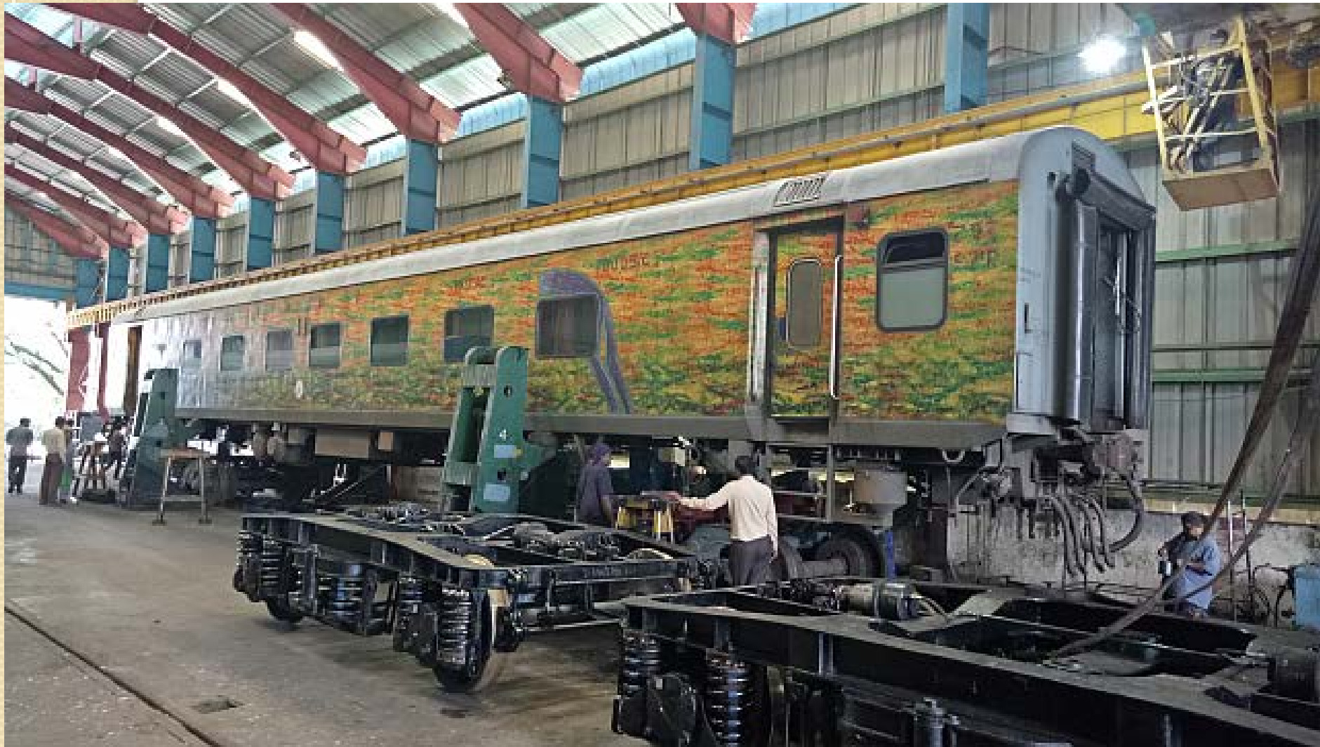
LHB coach in lifted condition (SS-1)
