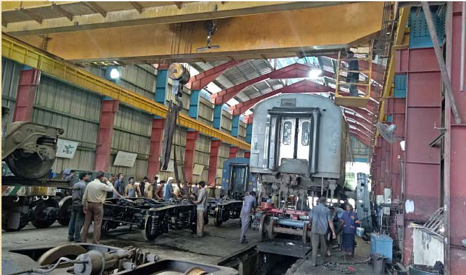
IOH shed, coaches in lifted condition on jacks
