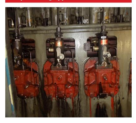
Unit injector consists of Bush and plunger type pumping arrangement in GM
