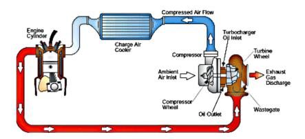
Initially Gear driven by Engine and thereafter driven by Exhaust gases
