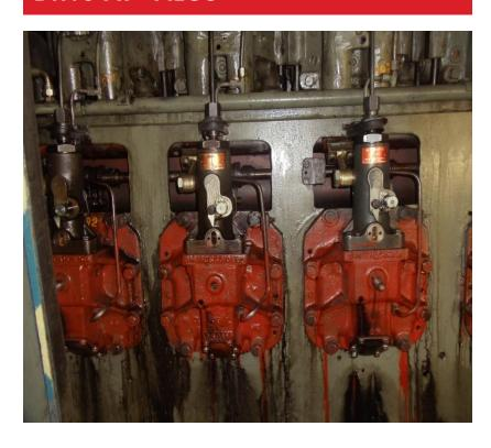
No High pressure tube, Rocker arm directly driven by Cam Shaft -GM
