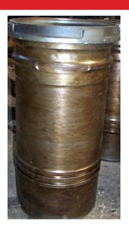
Laser hardened, In built water jacket, Air port for Air intake
