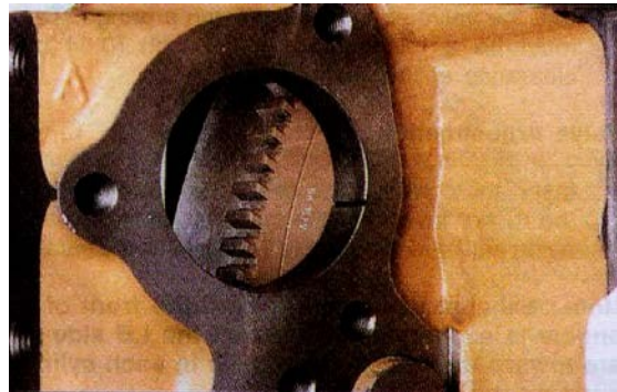
VS Mark on right bank flywheel
