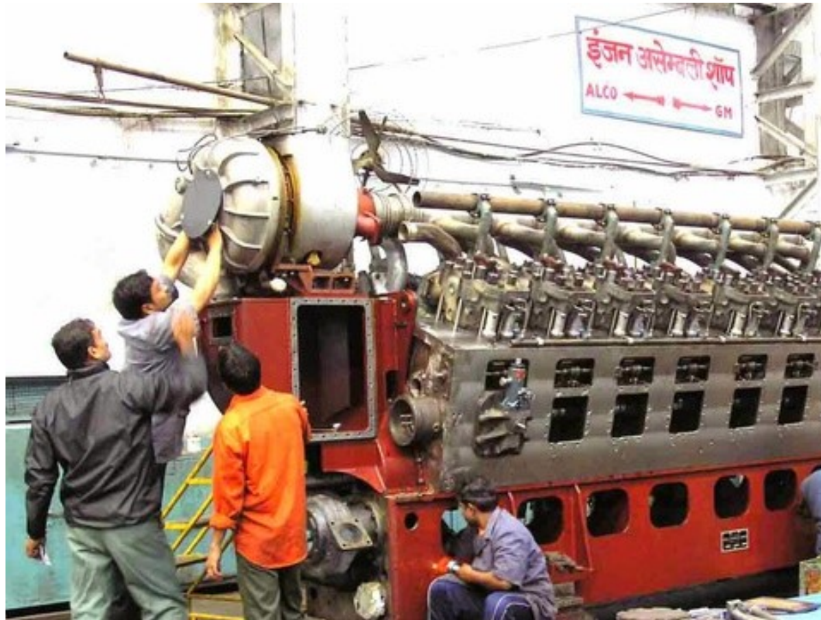
Diesel Loco Engine Block & its Components under fitment
