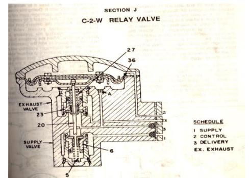
**C<sub>2</sub> W – Relay VALVE:** It is similar to C<sub>2</sub> relay valve with some additional features. It is connected to the BP charging/ exhausting system. It gets pilot air from A9 brake valve and it charges/ exhausts BP
