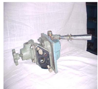
application of loco and formation brake. In release condition it charges BP up to 5.0 Kg/cm<sup>2</sup>(max). The BP pressure can be varied by moving its handle.
