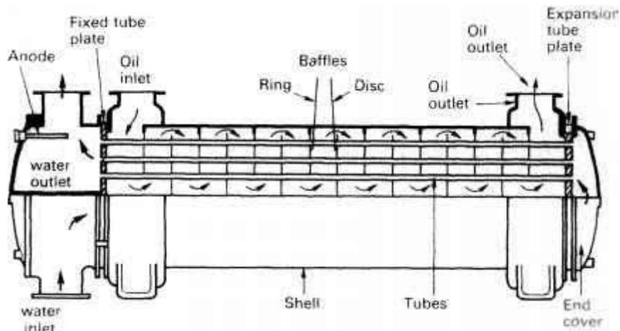
SHELL AND TUBE TYPE LUBE OIL COOLER
