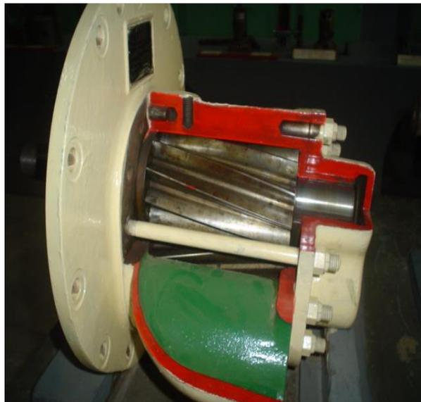
LUBE OIL PUMP (cut section)
