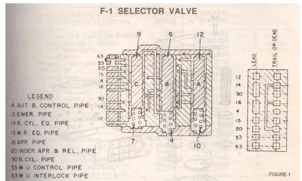
In co-ordination with MU2B, this valve makes the system to operate as a lead unit or trail unit.
