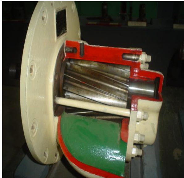
LUBE OIL PUMP (cut section)
