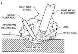
PROCESS USING BARE ELECTRODE & GASEOUS SHIELD
