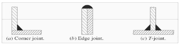
Each type of joint has its own symbol. The basic weld symbols are shown below:
