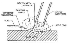
PROCESS USING FLUX COATED ELECTRODE
