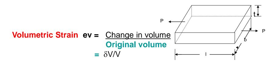
Bulk modulus: The ratio of the direct stress intensity to the volumetric strain within the elastic limit is known as bulk modulus. It is denoted by 'K'.
