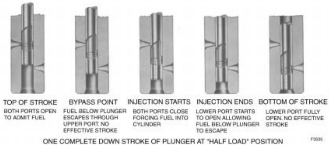
Figure 11-4. MUI Injector Fuel Flow
