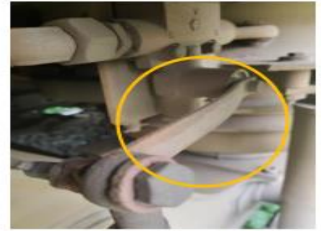
Resulting in -Leveling valve Handle in bent condition
