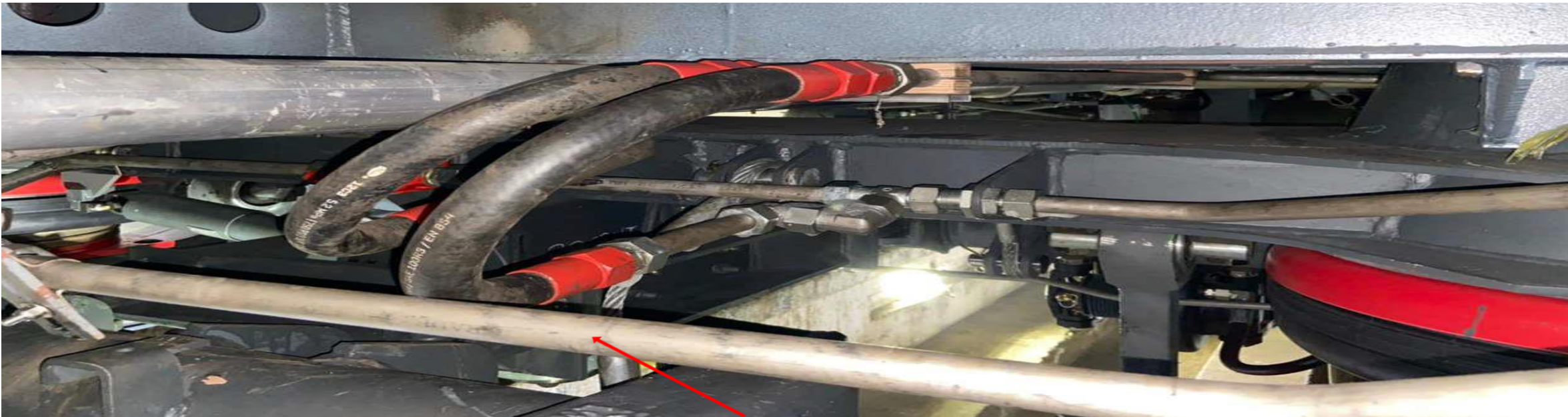
STEEL PIPE FOR CONNECTING FLEXIBLE HOSE PIPE TO LEVELLING VALVE
