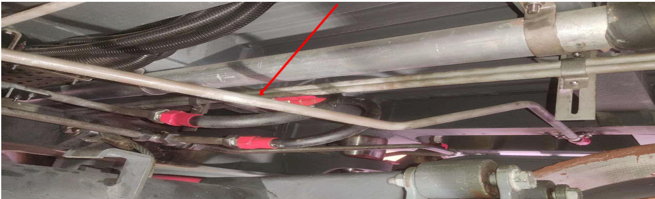
STEEL PIPE FOR CONNECTING FLEXIBLE HOSE PIPE TO LEVELLING VALVE
