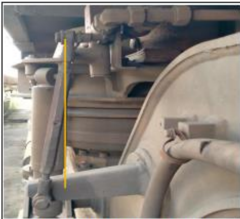
Improper Welding of Brackets
