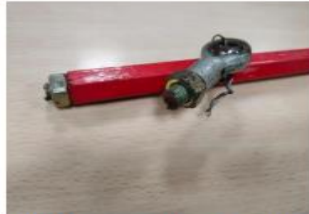
Resulting in -Installation Lever Broken
