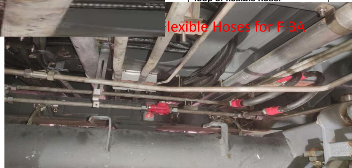
New pipe provided for smooth loop of flexible hose.
