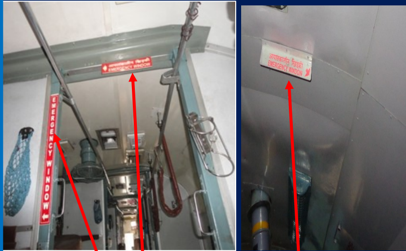
Location in coach indicated with fluorescent signage
