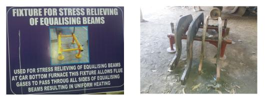
Proper stress relieving is done by providing a gap between the equalising beams thereby allowing the hot gases to contact with entire surface area of the beams. This ensures uniform heating of surface area and effective soaking. This also reduces the heat loss as well as the fuel consumption. This practice can be adopted in all over Indian Railways for the better results of heat treatment process.
