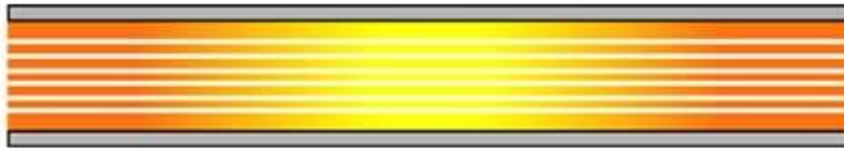
Laminar flow profile (Reynold's number \leq \sim 2300 )
