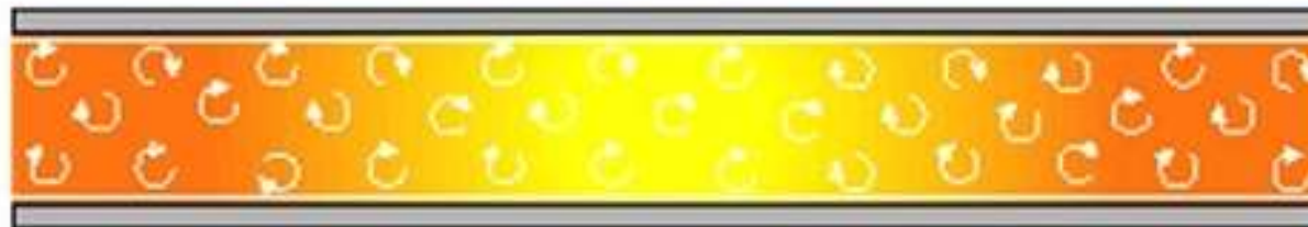
Turbulent flow profile (Reynold's number \geq \sim 3000 )
