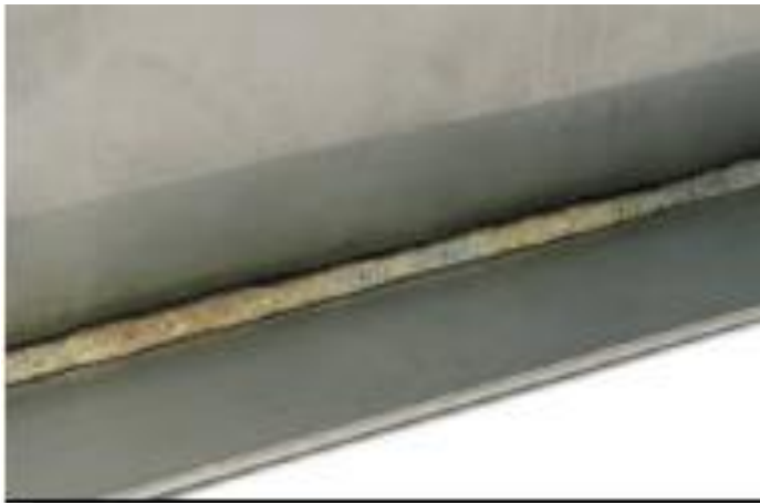
Application of short arc transfer
