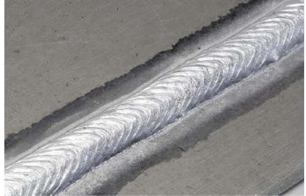
An aluminium weld done with the GMAW process
