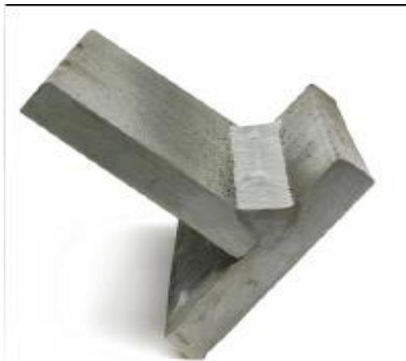
Application of axial spray arc transfer
