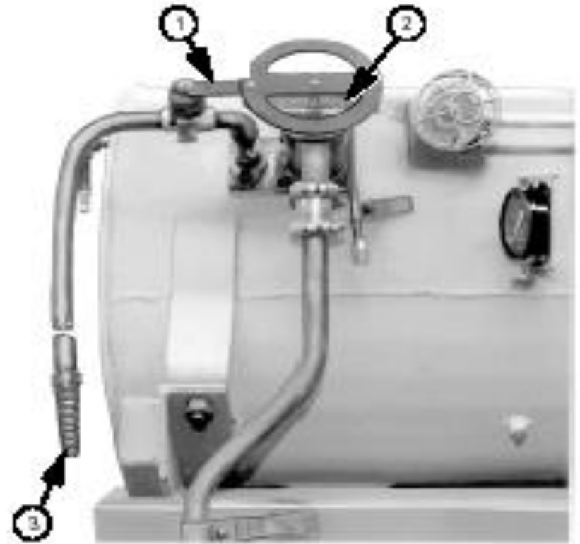
1. Filler/Relief Valve Handle (Pull Down To Open) 2. Pressure Cap 3. Filler Pipe Connector
