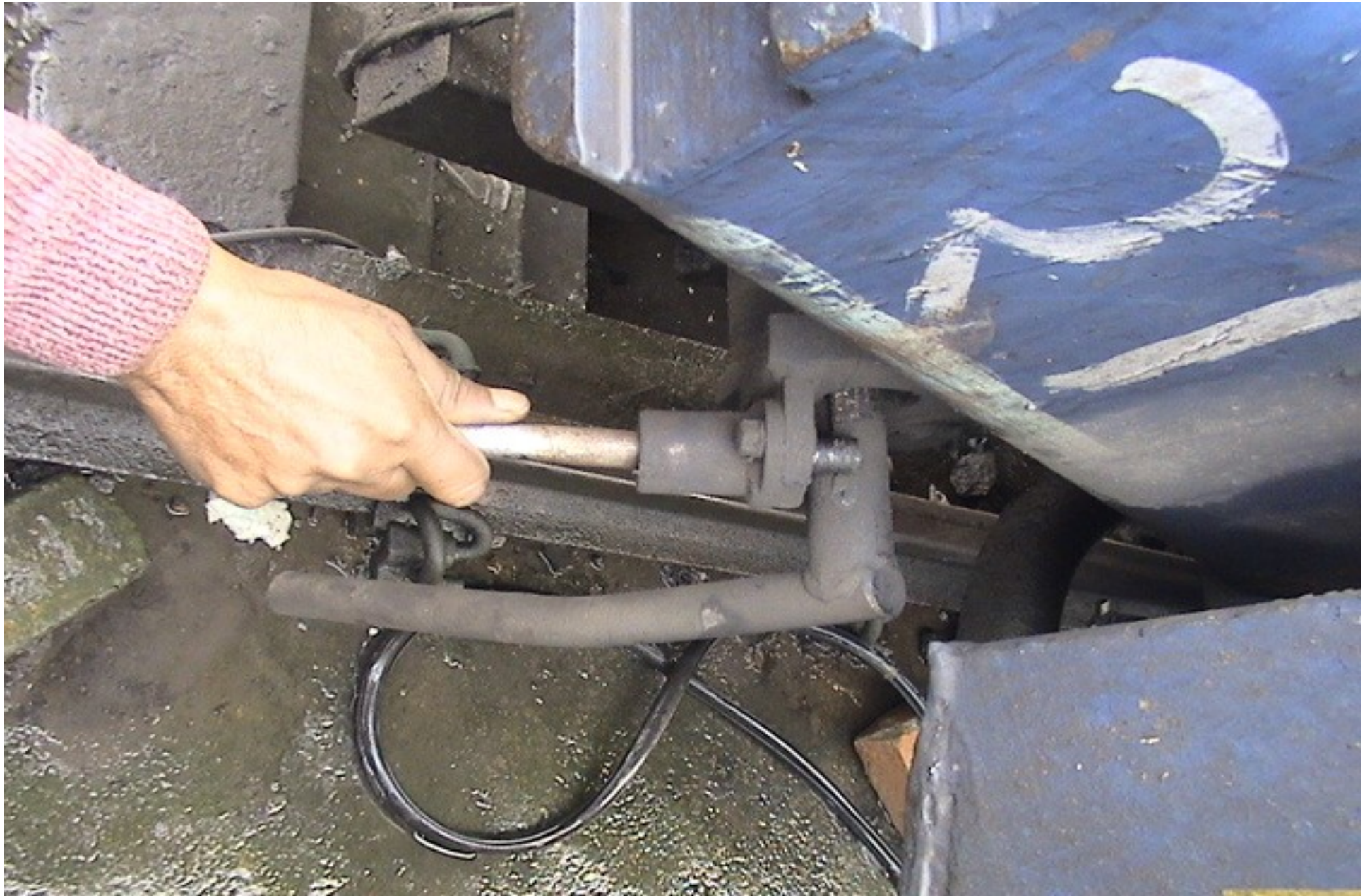
Manual Locking & Unlocking of Coupling Device
