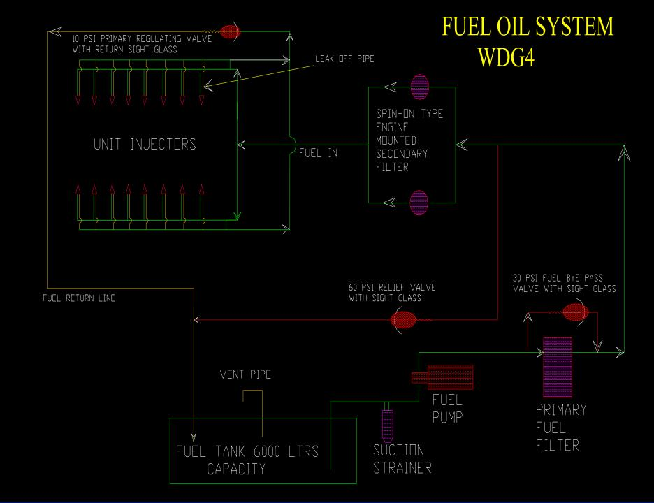
Fuel oil system is designed to supply fuel oil to the engine in correct quantity, correct pressure and at the right time according to the engine requirements.
