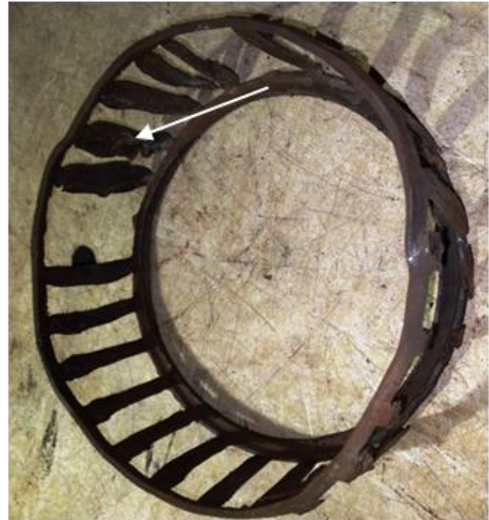
Fig.2- Showing broken & damaged cage
