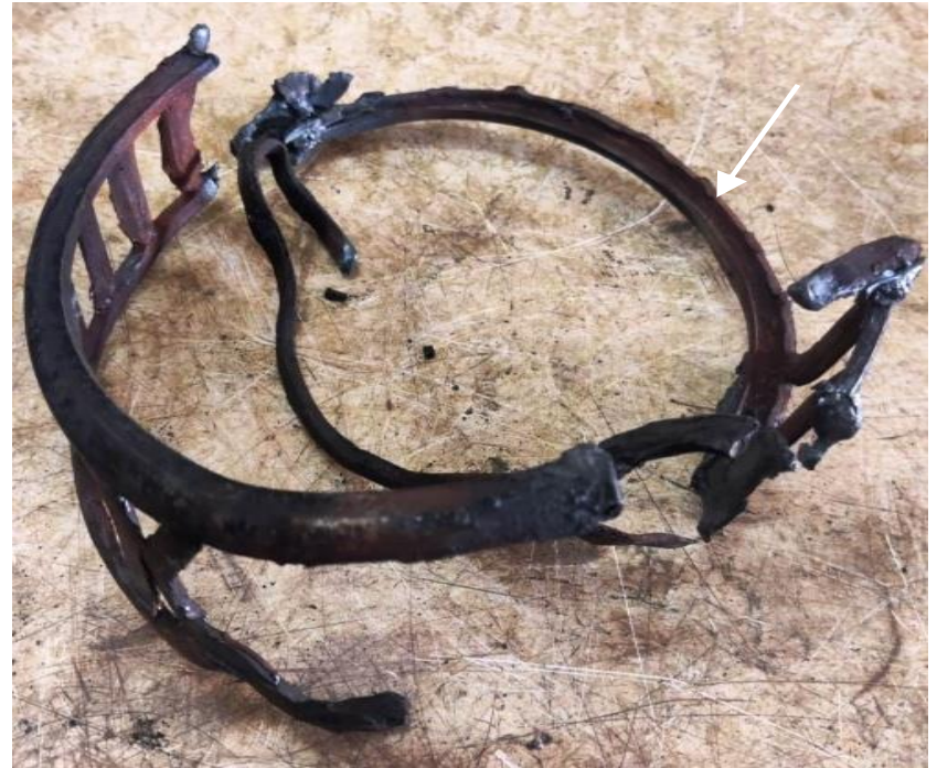
Fig.2- Showing broken , damaged & deformed cage
