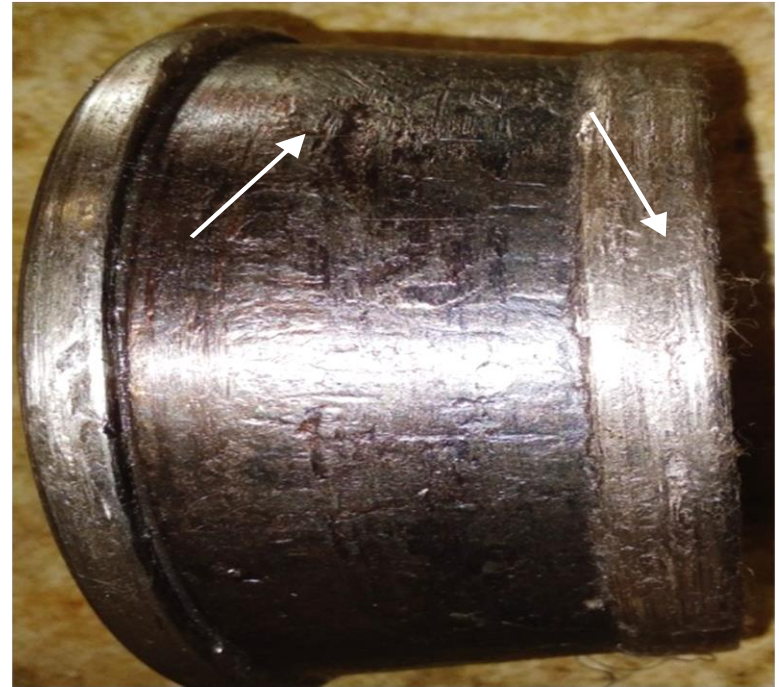
Fig.3- Showing plastic flow, wearing & flaking on outer surface of other cone.
