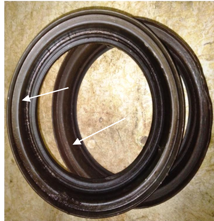
Fig.3- Showing one seal with rubber & contaminated grease and other seal without rubber.
