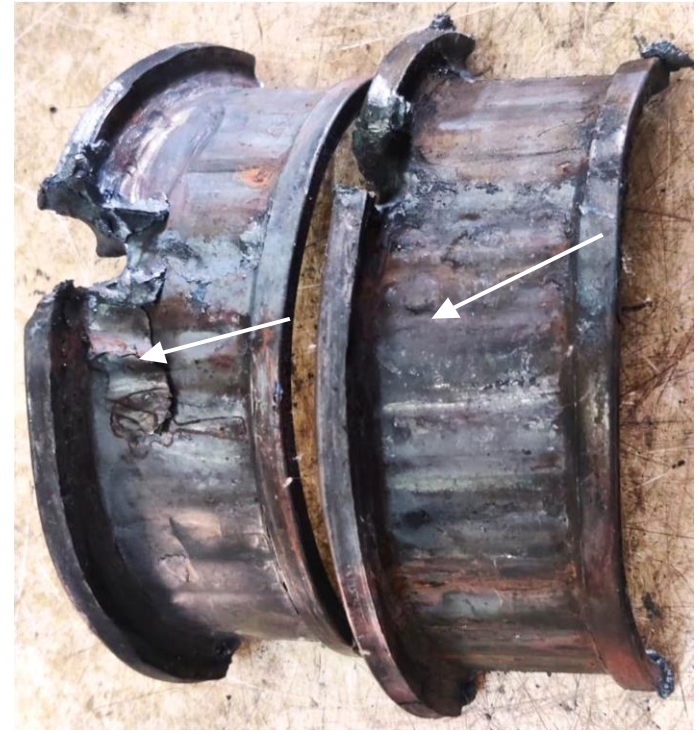
Fig.3- Showing deep brinelling marks with plastic flow of metal on outer surface of one of the cone.
