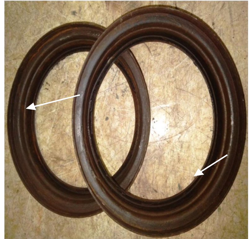
Fig.3-Showing both seals without rubber.
