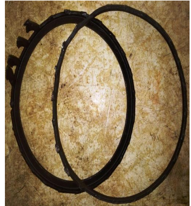
Fig.2- Showing broken & damaged cage.
