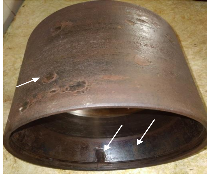
Fig.1- Showing pitting marks on outer surface and spalling, heat discoloration & brinelling mark on inner surface of the cup.
