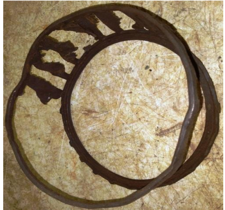
Fig.2- Showing broken, deformed & damaged cage.
