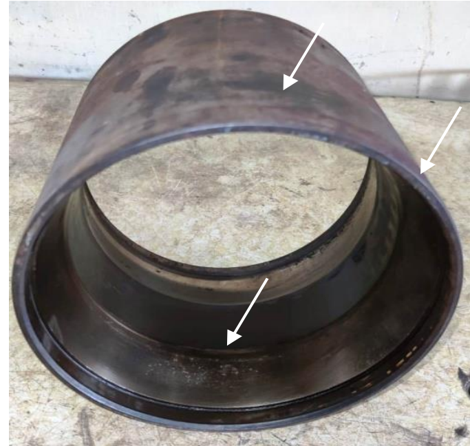
Fig.1- Showing Circumferential scoring on outer surface of cup. Spalling of metal and contaminated grease inside the groove on the inner surface of the cup and bulging at the edge of the cup.
