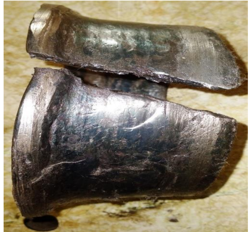
Fig.2- Showing one of the broken & heavily damaged cone.
