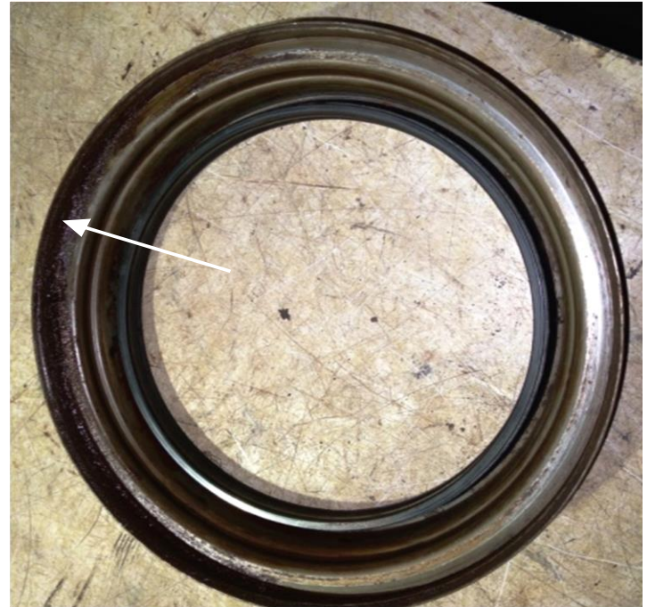
Fig.3- Showing contaminated grease on inner surface of the seal
