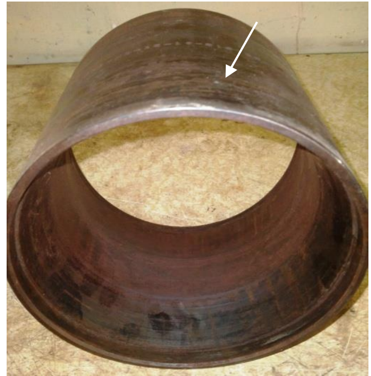
Fig.1- Showing scoring mark on outer surface of the cup.
