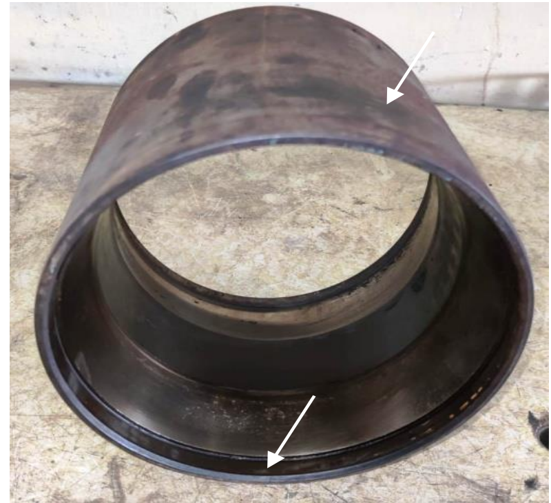
Fig.1- Showing circumferential scoring marks on outer surface of the cup and contaminated grease inside the groove.
