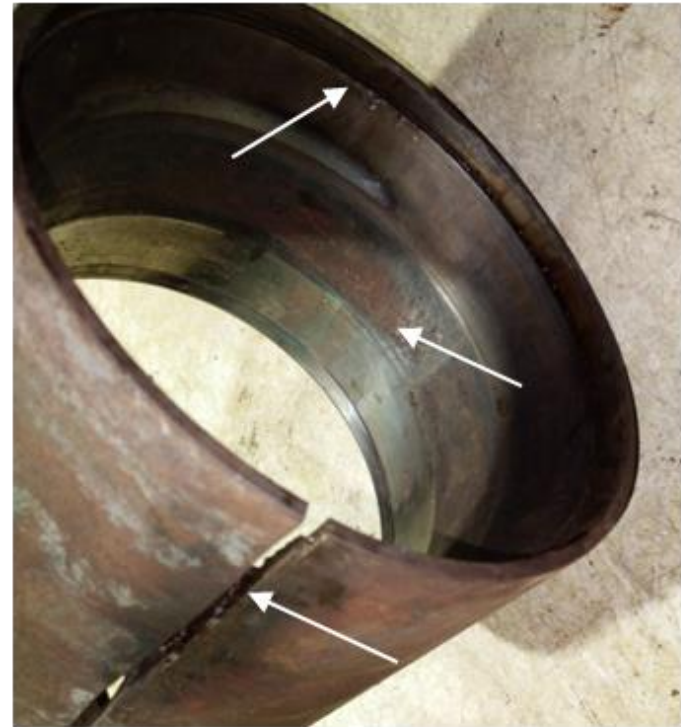
Fig.1- Showing longitudinal tearing , contaminated grease & spalling of metal on the Cup
