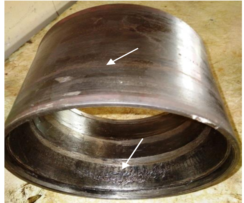
Fig.1- Showing scoring on outer surface and spalling & flaking on inner surface of the cup.
