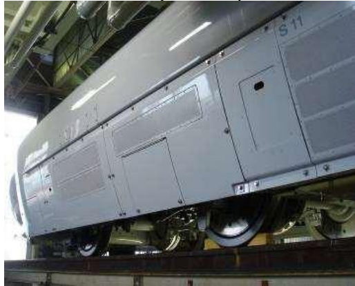
Bogie covers Sound-absorbing construction
