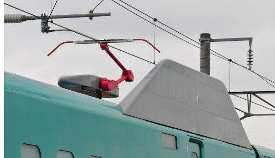
Pantograph noise insulation panel
