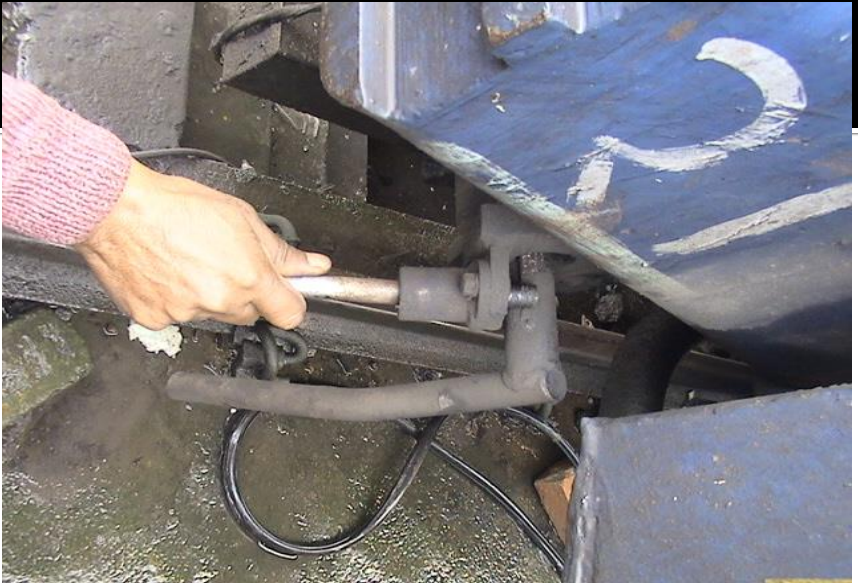
Locking and unlocking of manual uncoupling device
