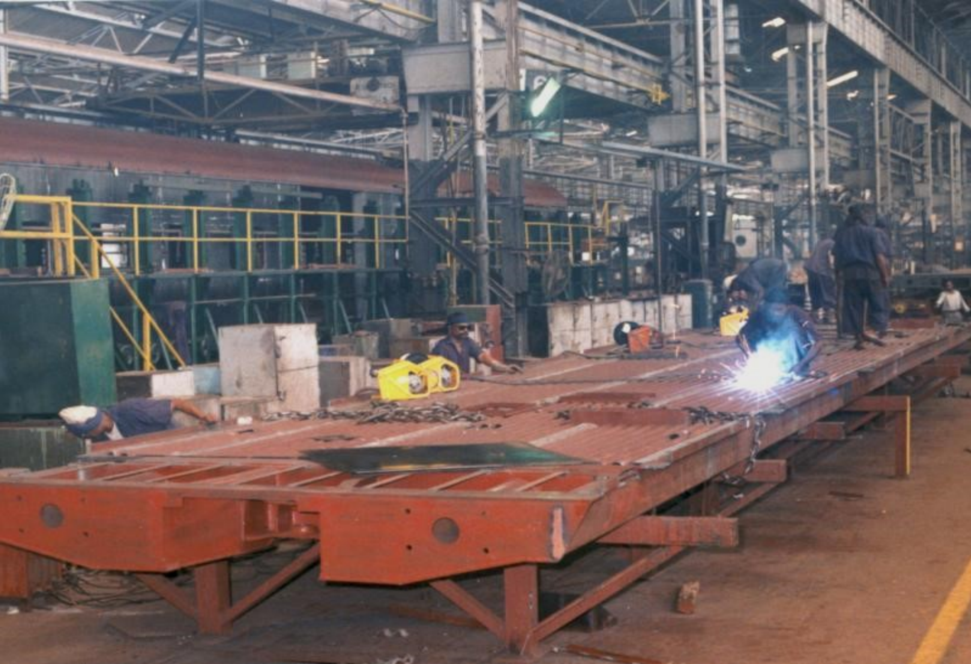
UNDER - FRAME WELDING
