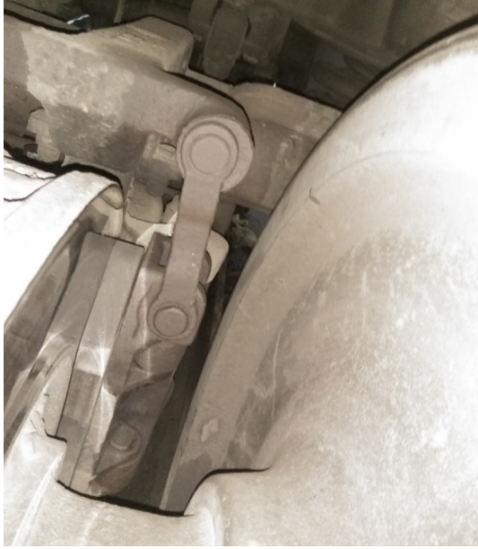
Lubrication of Brake Callipers
