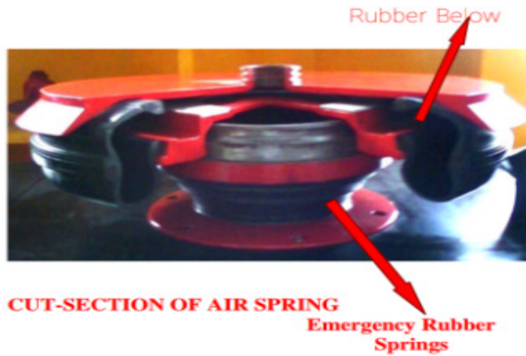
Schematic diagram of Air suspension
