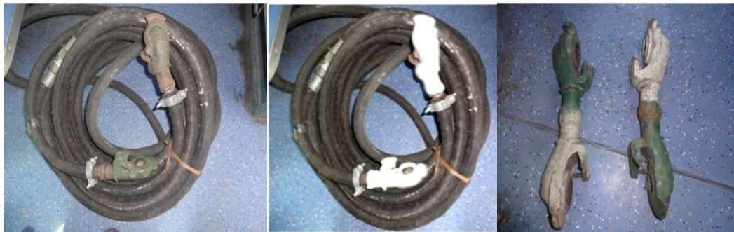
BP Coach Length flexible pipe FP Coach Length flexible pipe BP/FP by pass couplers
