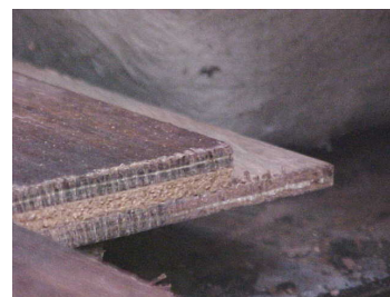
Flooring boards – Cork Sandwiched between COMPREG to absorb noise
