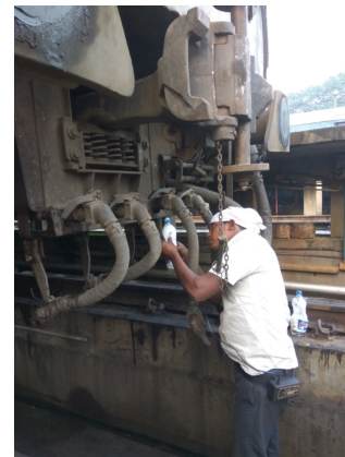
Check for air leakages at joints by means of soap solution
