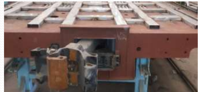
Provision for CBC as well a side buffer mounting in head stock
