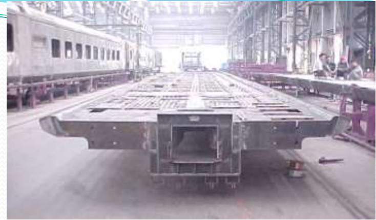
Provision for CBC as well a side buffer mounting in head stock
