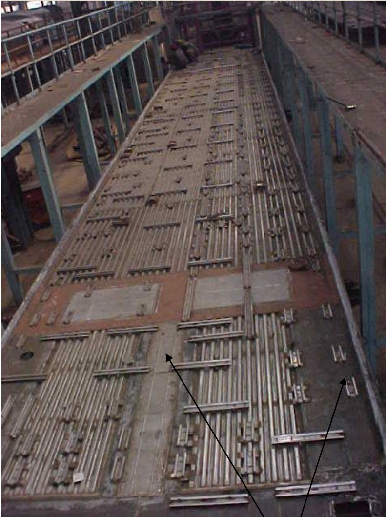
Flooring Support Members On Underframe
