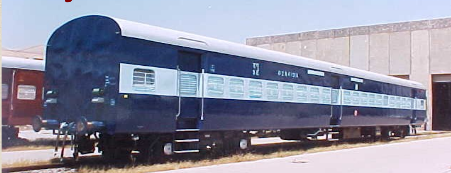
Corten steel Conventional coach - First coach turned out by RCF in March 1988
