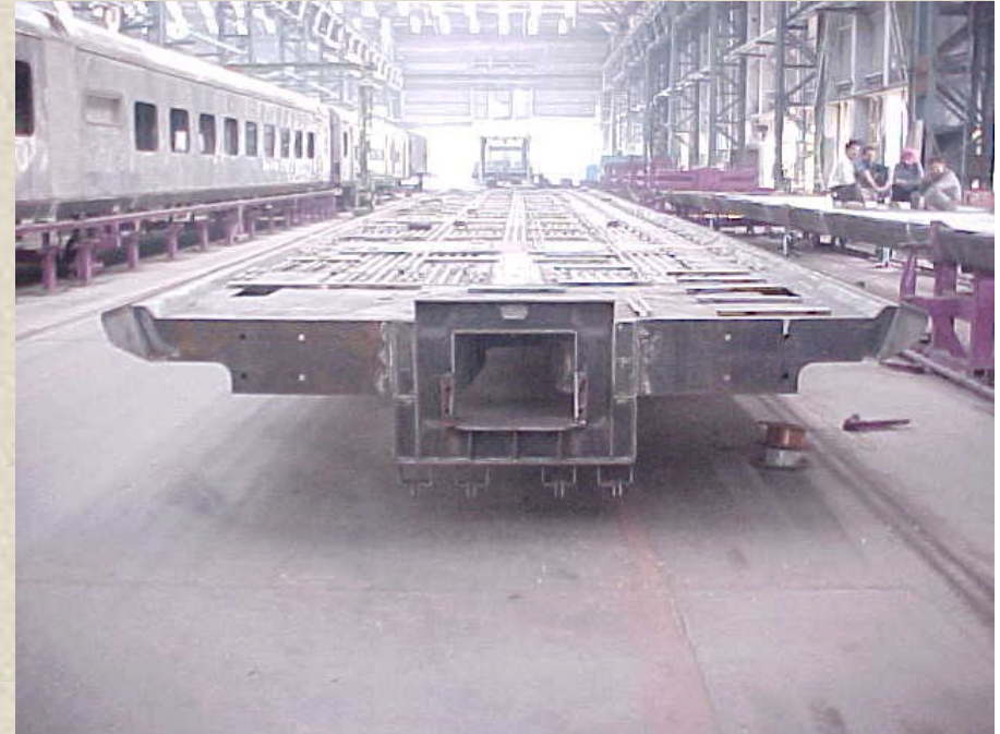
Provision for CBC as well a side buffer mounting in head stock
