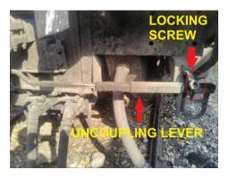
✓ Check CBC tell tale recess in coupled position, it should be clear and check for positive locking pin whether it is inserting in the tell tale recess or not.
