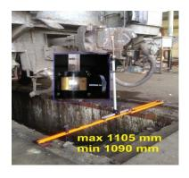
✓ Check the CBC of the power car and ensure its proper working. Close the knuckle and check whether the lock is falling freely. Observe full dropping of rotary lock assembly and proper sitting of uncoupling lever in the bracket. Ensure the rotary lock rib vertically downwards.
