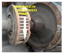
$\checkmark$  If any of the above defects are found, mark the coach sick for replacement of wheel along with disc.
