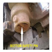
Check the uncoupling device lever with rotary lock and its sliding rod for any bent. Check bolts and nuts of mounting bracket for breakage / slackness, if so attend them.
