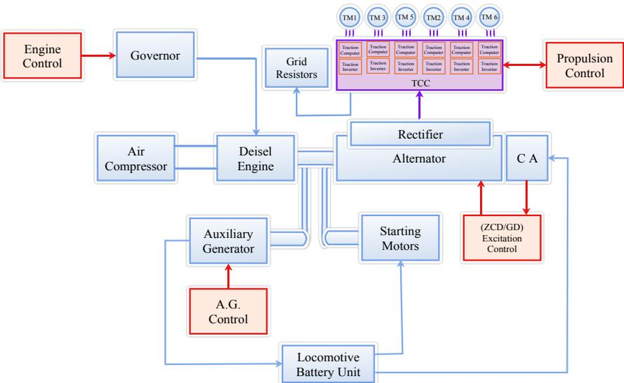
Fig. 1.2 Block Diagram of Locomotive Control System
