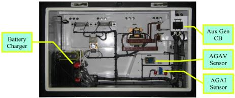
Fig. 5.3 Internal View of ECC#2
