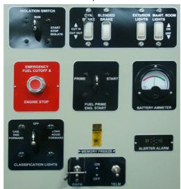
Fig. 5.10 Engine Control Panel
