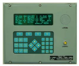
Fig. 11.1 Display Panel Keypad
