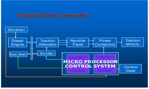
Medha's Microprocessor Based Locomotive Control System MEP 660 overcomes all the limitations of conventional locomotives. It also provides a superior control mechanism, protection to traction equipment, fault diagnostics, and adaptability to different engine types, flexibility in system configuration, etc.
