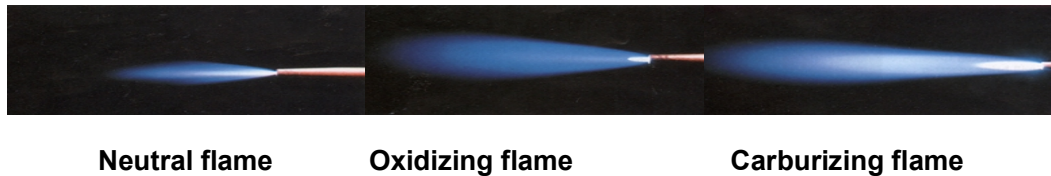
Fig 8: Different flames produced by controlling the gas flow
