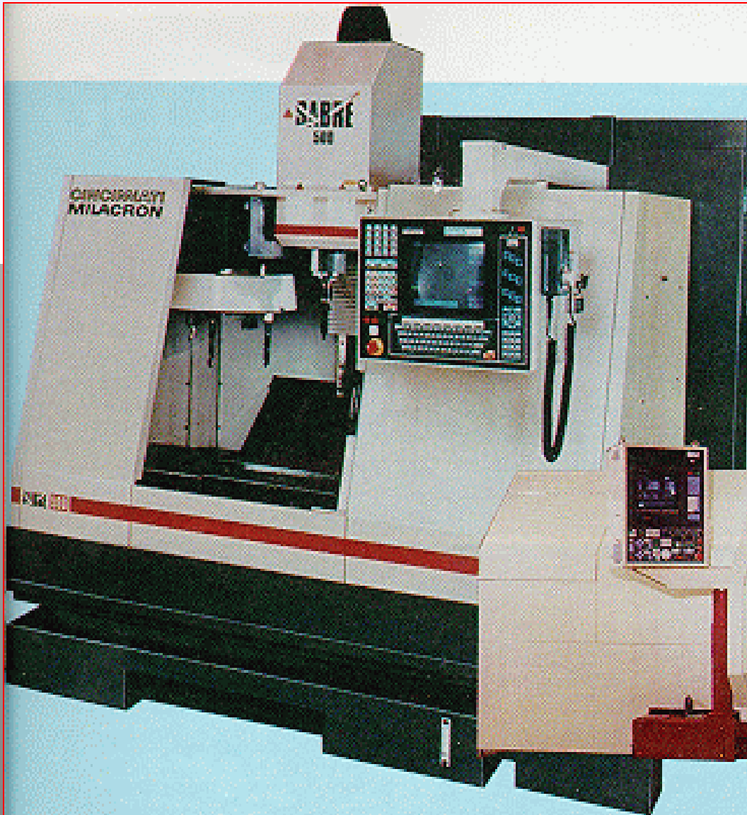
Fig. 12. Vertical machining center.
